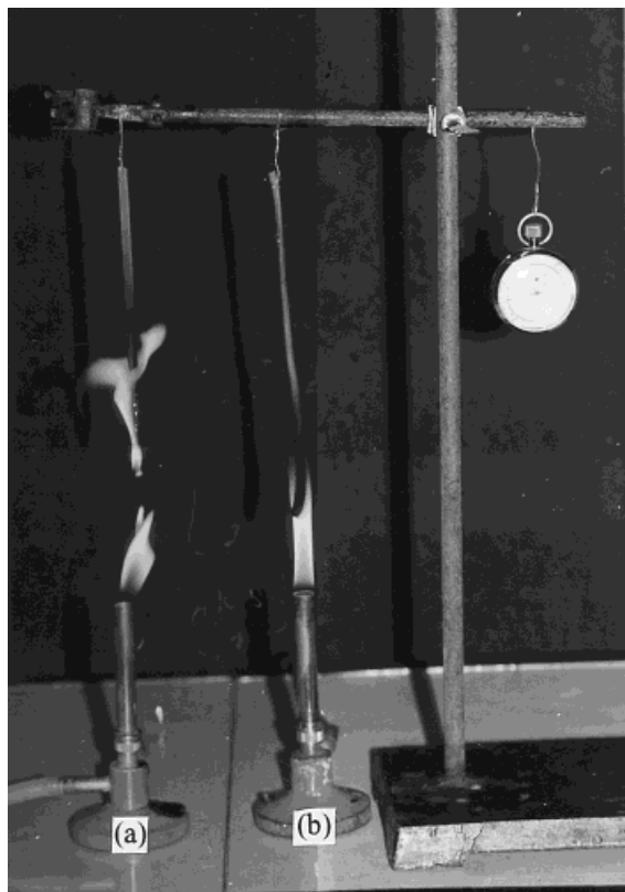
Figure 14 Vertical burning test. (b) Experimental sample with (a) a control after firing for 10 s.
